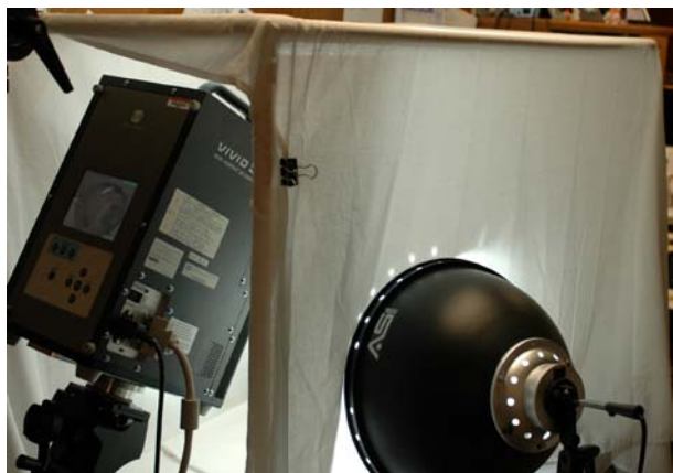
Figure 6. Light tent with scanner array.
