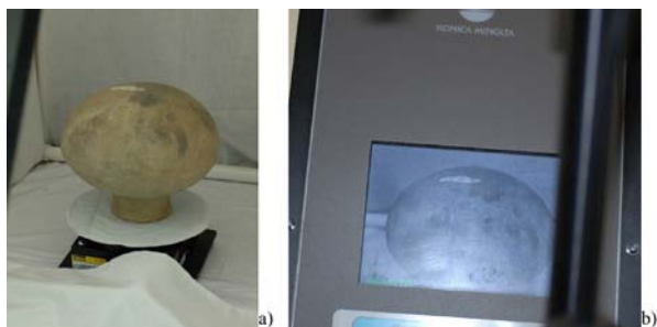
Figure 2. Artifact placed on computer-controlled turntable (a). Artifact as seen through scanner viewfinder (b).
