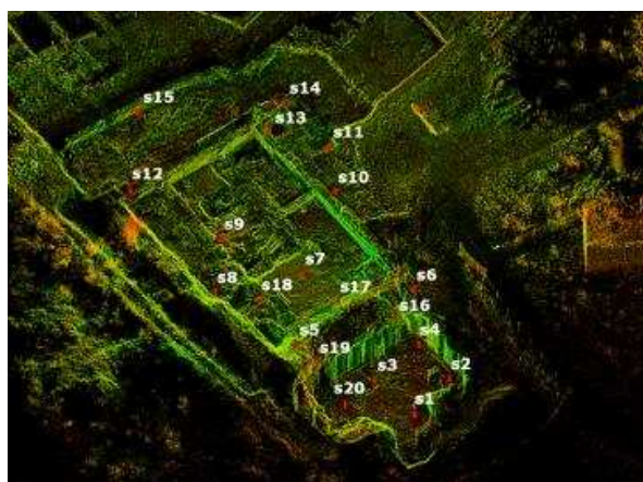
Figure 7. Topographical network for the laser scanning stations.
